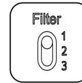
Filter 1 (off position) standard half band digital filter.
